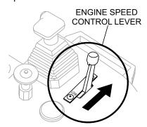
Figure 12. Engine Speed Control Lever (High)
